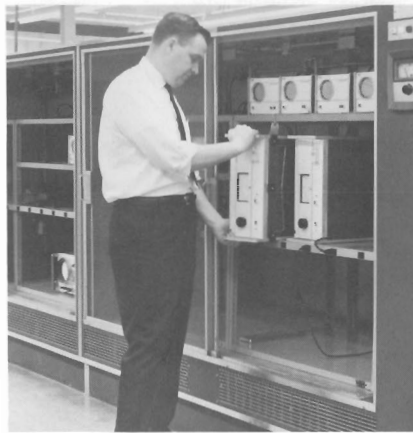
Uncovering weaknesses in products before they get into the hands of customers is the function of this aging cabinet designed by Waltham's Dick Meaney (above). Instruments get 15 hours of fast aging to expose hidden problems.
