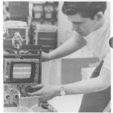
Shaker test at Colorado Springs is another way divisions are catching faults before they turn into costly warranty claims. Most such problems occur early in the life of an instrument. Here, Leon Skidmore tests new oscilloscope.
