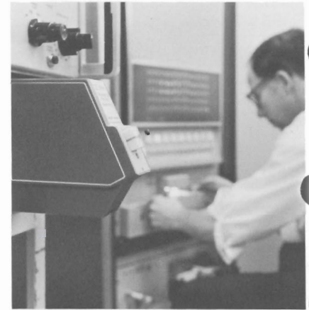
Components can be prime source of after-sale trouble, particularly when exposed to loads not contemplated in specs. Here, Microwave's Terry Bowman conducts computer-based test of parameters of transistor seen in foreground.
